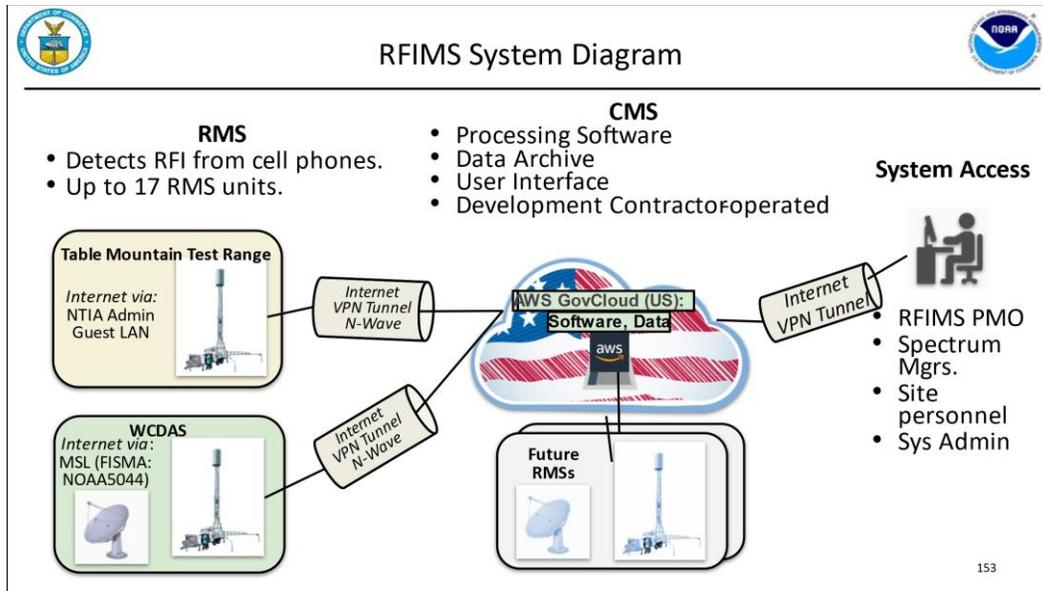
He noted that up to 17 RMS units can be deployed. They would all be connected to the Central Monitoring System. In the future, the CMS will be used by Spectrum Managers and other personnel.
